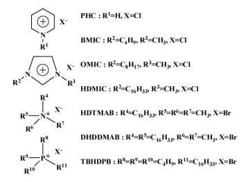
Fig. 2. Structures of various halide salts investigated in this work.
